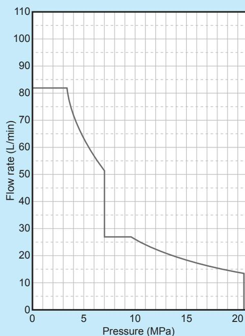
\* Operating flow rate at the maximum pressure in continuous operation: 14 L/min maximum
