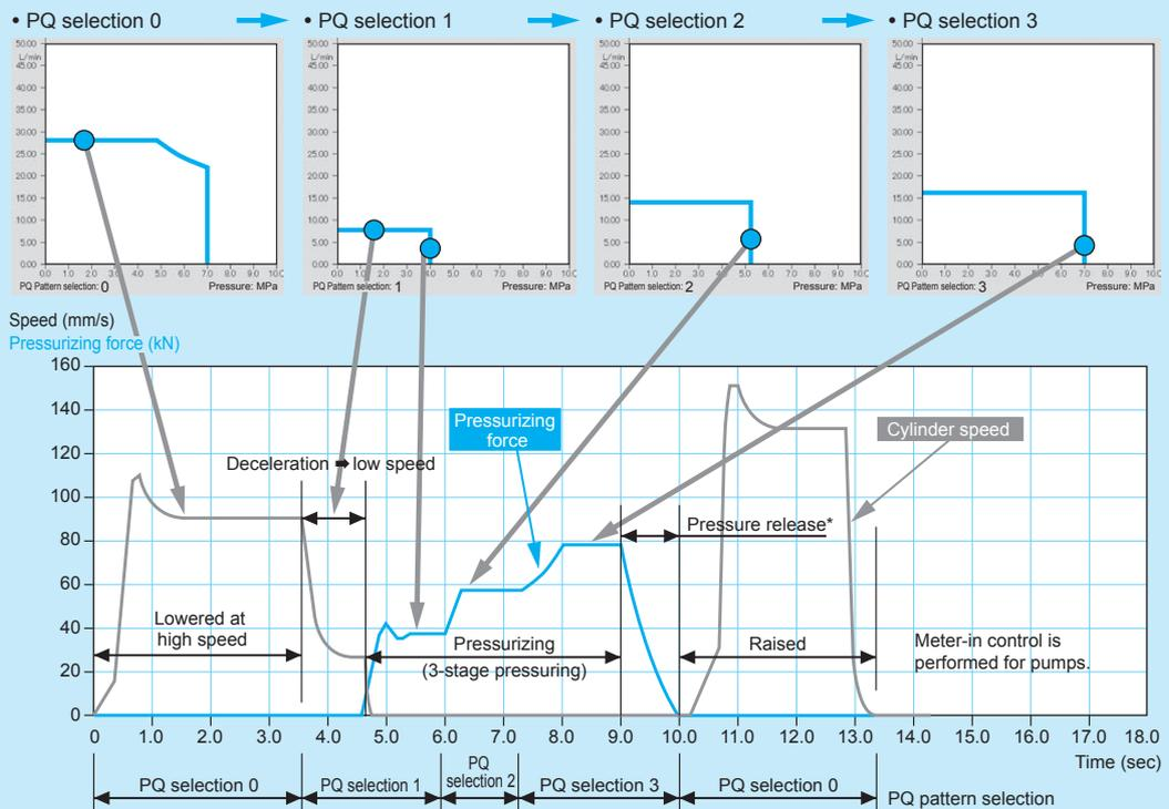
\*: When pressure release control is disabled, an additional pressure release circuit should be provided for the load side.
