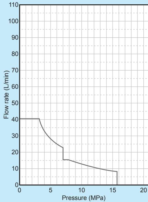
\* Operating flow rate at the maximum pressure in continuous operation: 8 L/min maximum
