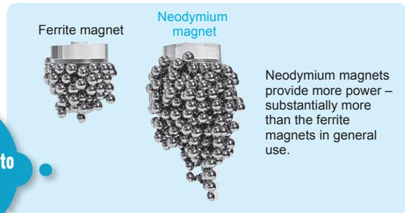
※1: A compound of neodymium (Nd, rare-earth element), iron (Fe), and boron (B). Neodymium magnets are known to have superior magnetic properties.
