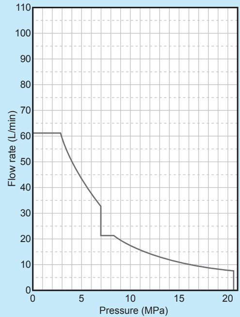
\* Operating flow rate at the maximum pressure in continuous operation: 6.5 L/min maximum
