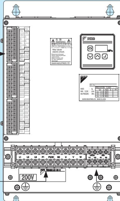
Solenoid valve terminal block (M4)
