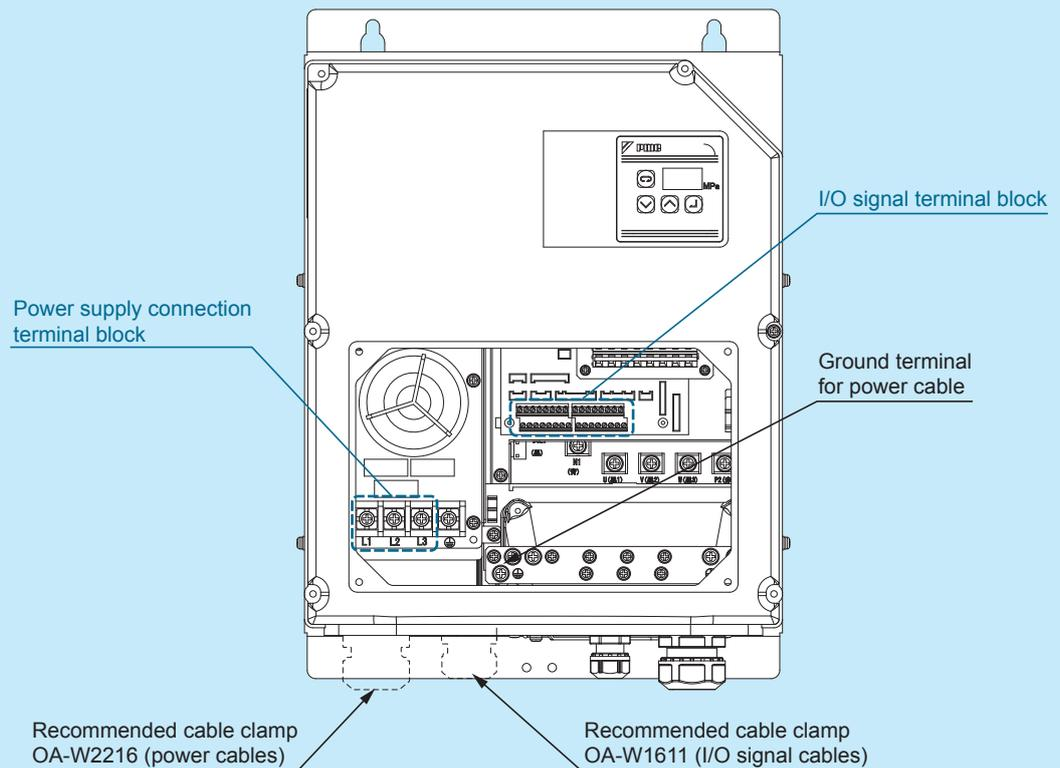
\* Main power supply connections: Connect a 3-phase AC power supply (200 V/50 Hz, 200 V/60 Hz, or 220 V/60 Hz) to the power supply terminals (L1, L2 and L3), and connect a ground cable to the ground terminal.
